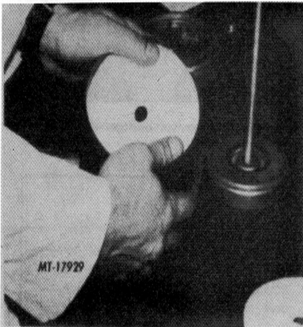
Fig. 10 Installing Felt Cloth In Cartridge
