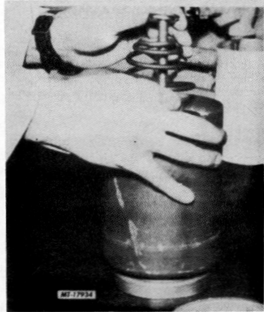
Fig. 15 Positioning Spring Retainer On Spring
